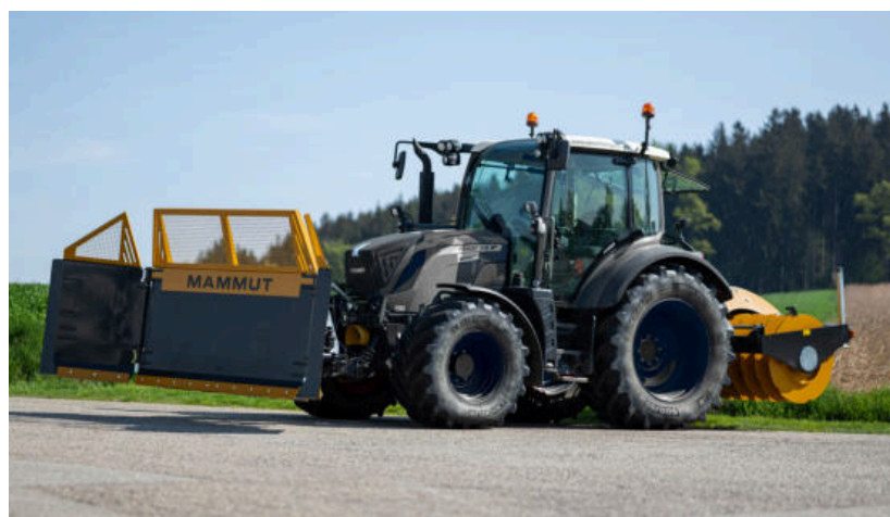
The ideal silage harvester for maize harvesting: Spreading and compacting in one work step
